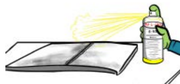
R-504 used as a penetrant remover. Spray on wiping media, and wipe remove penetrant.
